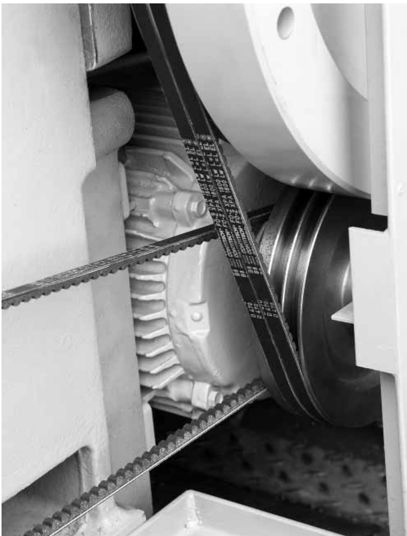
Matched length CONTI FO ® -Z heavy-duty raw edge V-belts on a paper-cutting machine
