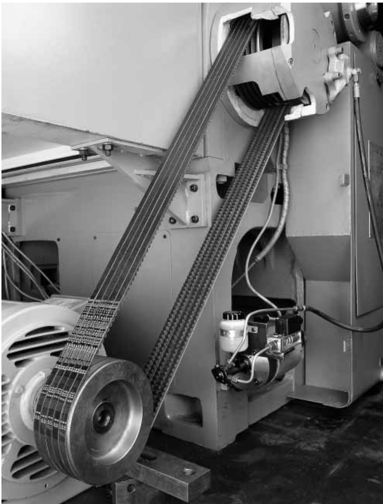
CONTI FO ® -Z heavy-duty cogged raw edge V-belts on a machine tool
